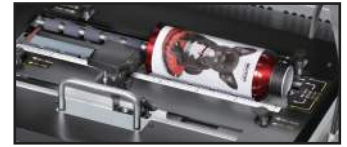
ROTARY UNIT Enables printing on cylindrical objects.
