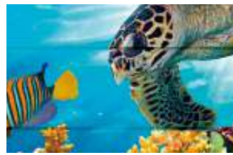
Overlap/Black streaks (Insufficient feeding amount)
