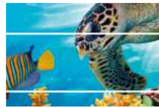
Gap/White streaks (Excessive feeding amount)
